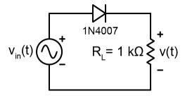
Use the function generator to provide a sinusoidal input signal  $v_{in}(t)$  with the following properties:
