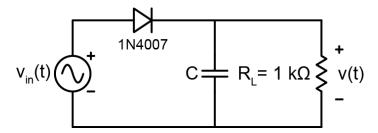
The role of the filter is to smooth out the ripple in the output voltage, thereby making the output voltage closer to an ideal DC source. Again, measure and record the output waveform v(t), for capacitance values of  $C = 1 \mu F$ ,  $22 \mu F$ , and  $220 \mu F$ .
