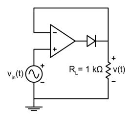
Measure and record the output voltage v(t) for both 60 Hz and 440 Hz input voltages.
