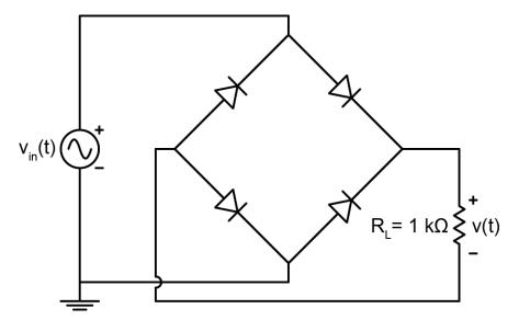
Note: In this circuit, the input signal  $v_{in}(t)$  and output signal v(t) do not share a common ground connection. (I.e., the rectified output signal is "floating".)
