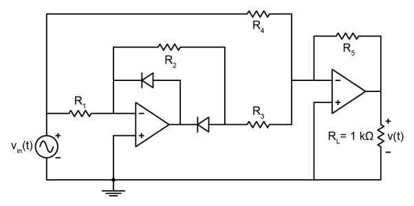
Simulate your circuit in PSpice and make a plot of the output voltage when the input voltage is a sinusoidal voltage with amplitude 8 Vpp and frequency 440 Hz. Submit a screenshot of your schematic, showing your design, and a simulation showing the input and rectified output.
